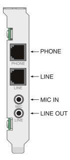
Figure 2-2. MT5634ZPX-PCI-V92 connectors.
